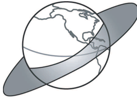
Figure 5.1. The shaded disc is that portion of the orbital plane lying within an inclined circular orbit. If the Earth did not rotate, the line where the shaded disc meets the Earth's surface would be the ground track of the satellite. This figure shows that, for an inclined orbit, the ground track passes above and below the equator.
